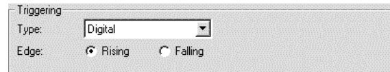
Digital Trigger With Digital Trigger, the user must indicate Rising or Falling Edge.
